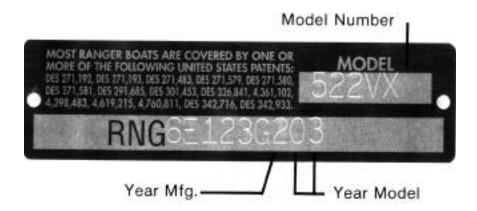
The hull I.D. Plate is located on the outboard side of the starboard transom, above the water line, and contains the following information:
