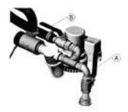
4. Close valve (A) when system is not in use.
