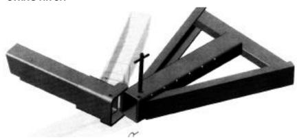
To operate the swing hitch, pull the pin out of the bottom of the T-handle pin, fold up the safety catch on the bottom of the T-handle pin, pull the T-handle pin out of the frame and the hitch can now be swung to the side. When returning the hitch to the tow position the T-handle pin and the safety pin must be installed. NEVER TOW YOUR TRAILER WITHOUT THE T-HANDLE PIN AND THE SAFETY PIN INSTALLED!
